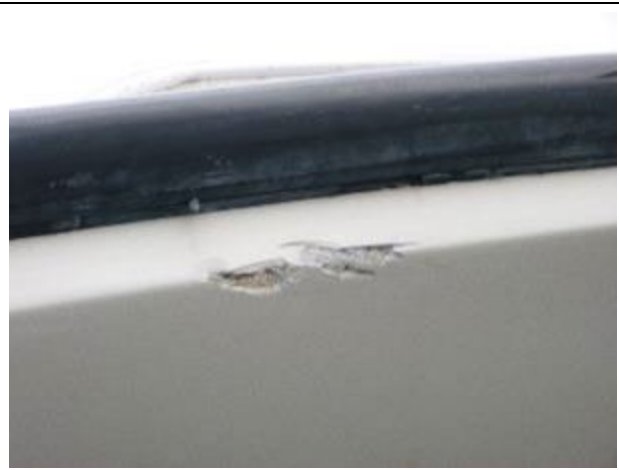
Numerous gelcoat gouges on the topsides.
