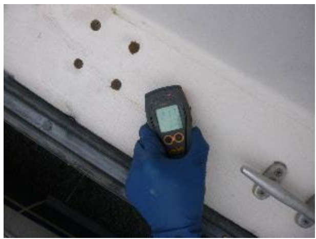
Elevated moisture in the starboard side deck. Meter reading 217.
