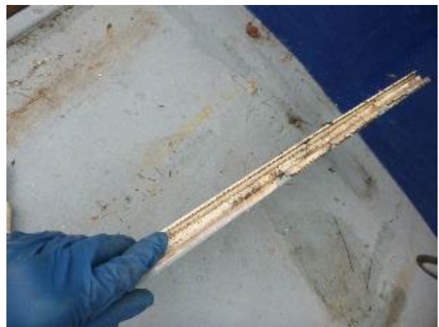
The lazaret hatch cover is missing its O-ring.
