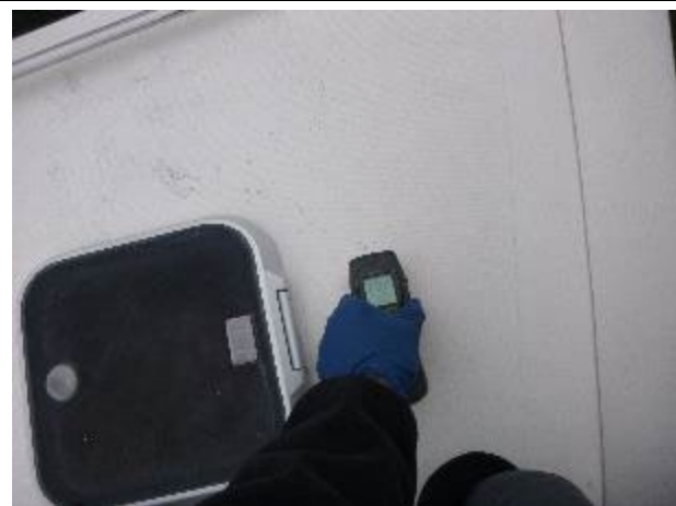
Elevated moisture in the starboard side of the forward trunk cabin. Meter reading 202.
