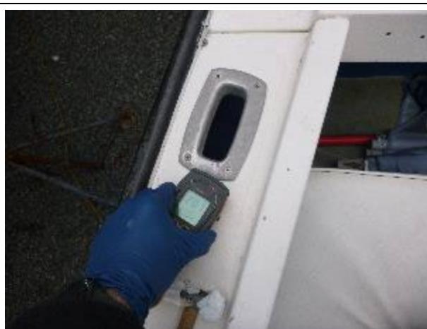
Elevated moisture in the starboard aft coaming top. Meter reading 207.
