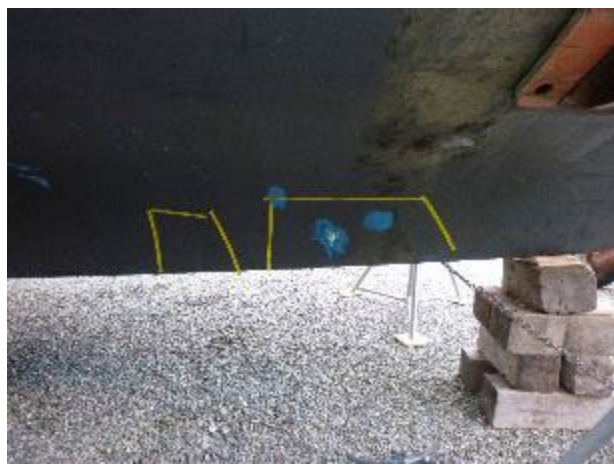
Yellow tape marking off areas of gelcoat stress cracking on the starboard keel.
