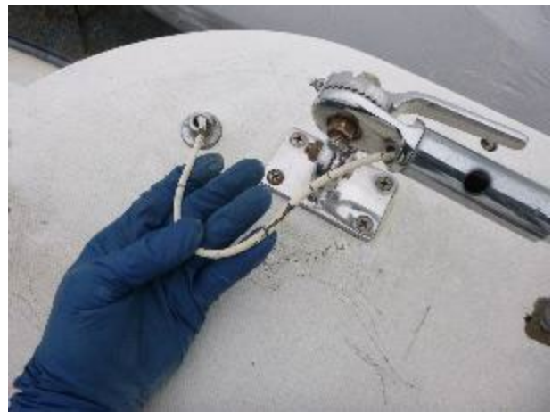
The starboard VHF antenna wire is deteriorated.
