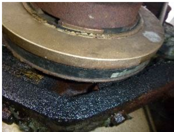
Signs of an oil leak near the forward crank shaft seal.
