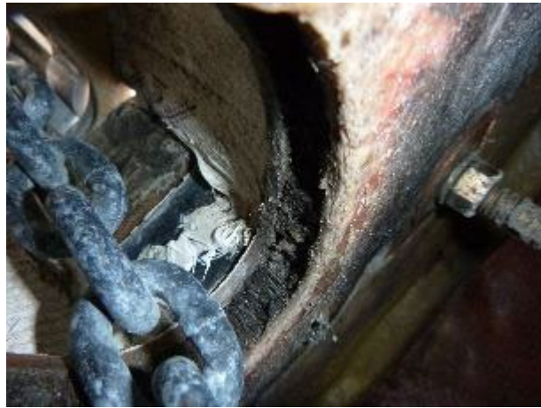
Deteriorated foredeck core at the anchor chain hawse pipe.
