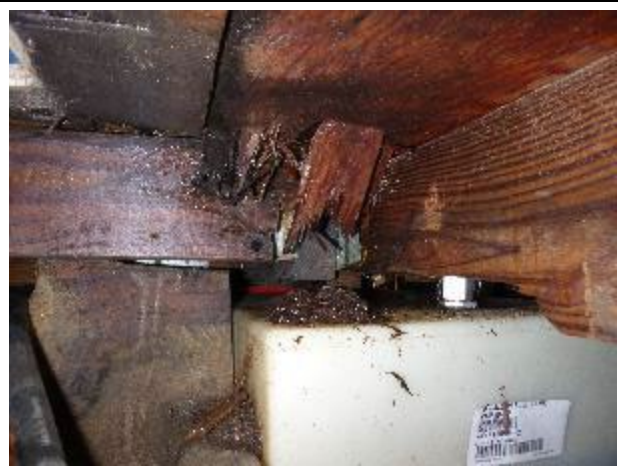
Cockpit sole plywood and structure deteriorated and wet aft of the starboard fuel tank.
