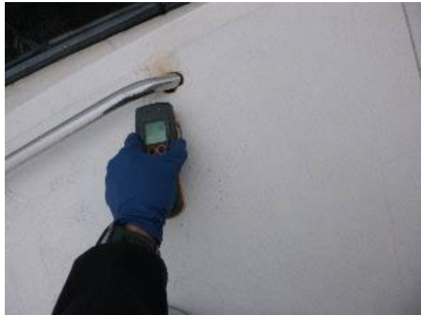
Elevated moisture in the starboard side of the forward trunk cabin. Meter reading 215.
