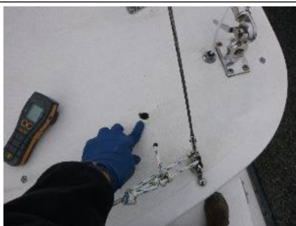
Elevated moisture in the starboard aft coaming top. Meter reading 207.
