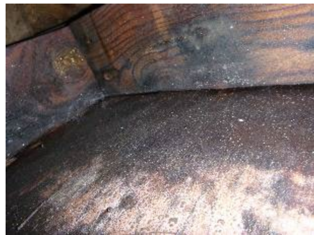
Cockpit sole plywood wet and starting to deteriorate aft.
