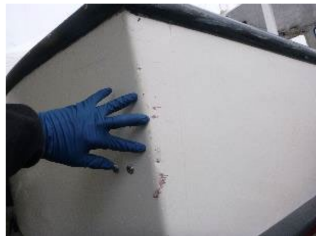
Transom corner damage.
