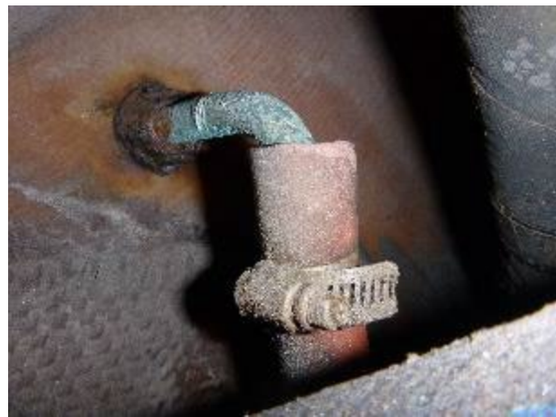
The vent fitting for the removed port fuel tank is deteriorated.
