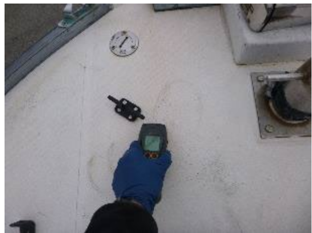
Elevated moisture in the foredeck. Meter reading 239.
