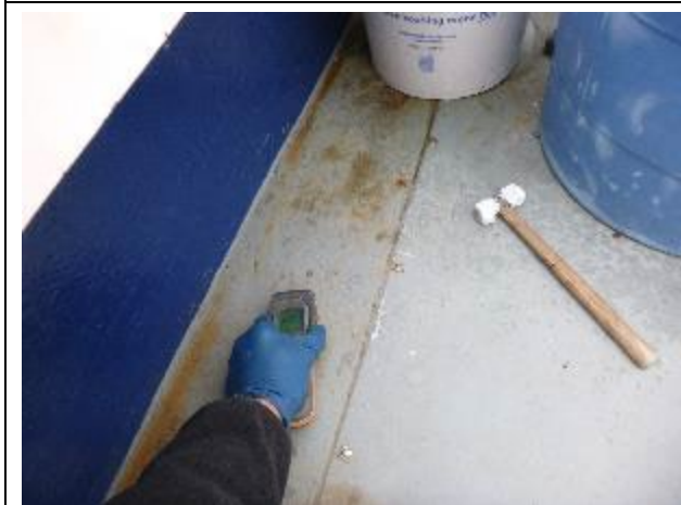
Elevated moisture in the cockpit sole to starboard of the engine box. Meter reading 207.
