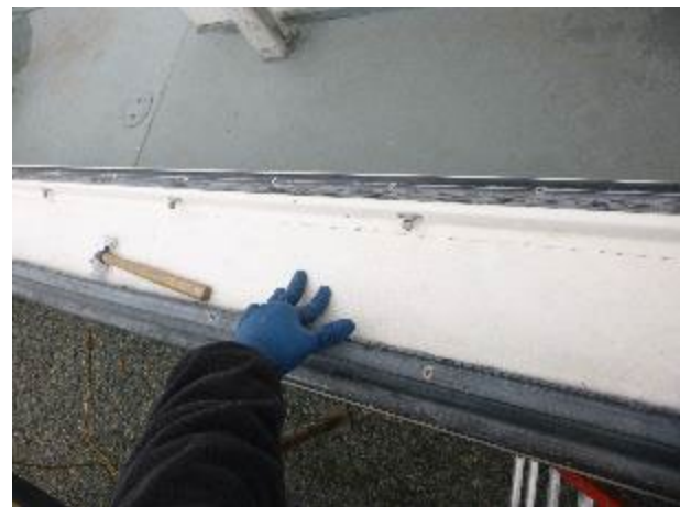
Delamination in the starboard cockpit coaming top.
