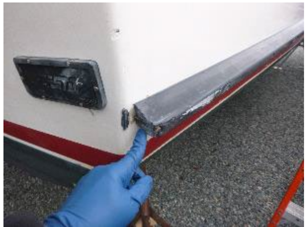
Starboard aft spray rail broken.
