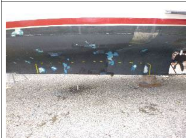
Yellow tape marking off area of gelcoat stress cracking the port amidships keel.
