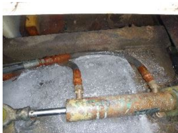
Steering hose ends rust at the steering ram.
