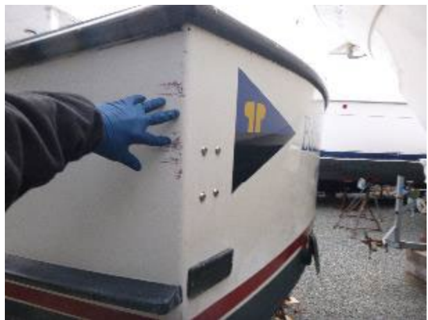
Transom corner damage.
