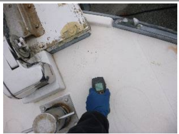
Elevated moisture in the foredeck. Meter reading 212.
