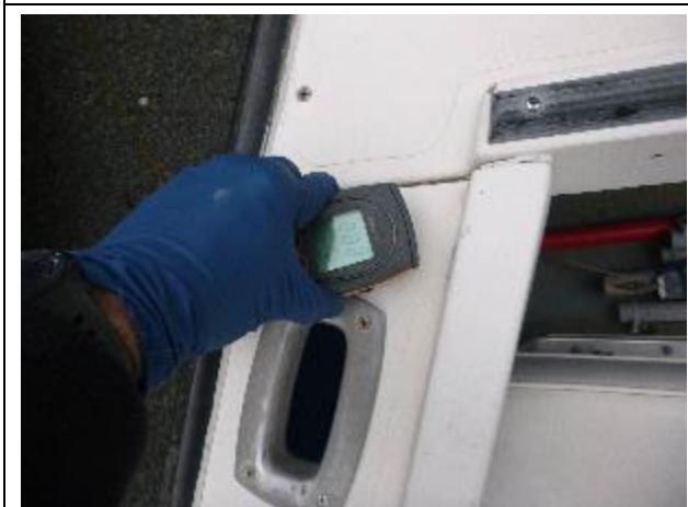
Elevated moisture in the starboard aft coaming top. Meter reading 202.
